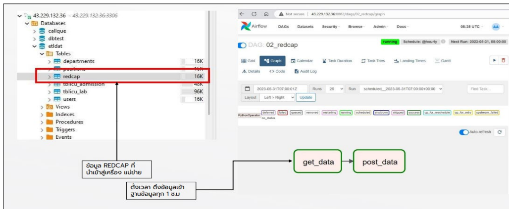
Fig. 3: Apache Airflow DAG illustrating workflow orchestration for REDCap data extraction, transformation, and loading.
