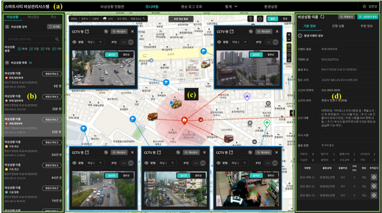
Fig. 3: Web-GIS dashboard configuration; (a) GNM for moving between menus, (b) Local navigation menu for searching emergency, CCTV footage, and address, (c) GIS map information such as emergency location, CCTV footage, and dispatch vehicle location, (d) Right panel menu for searching basic information, progress, and neighborhood information
