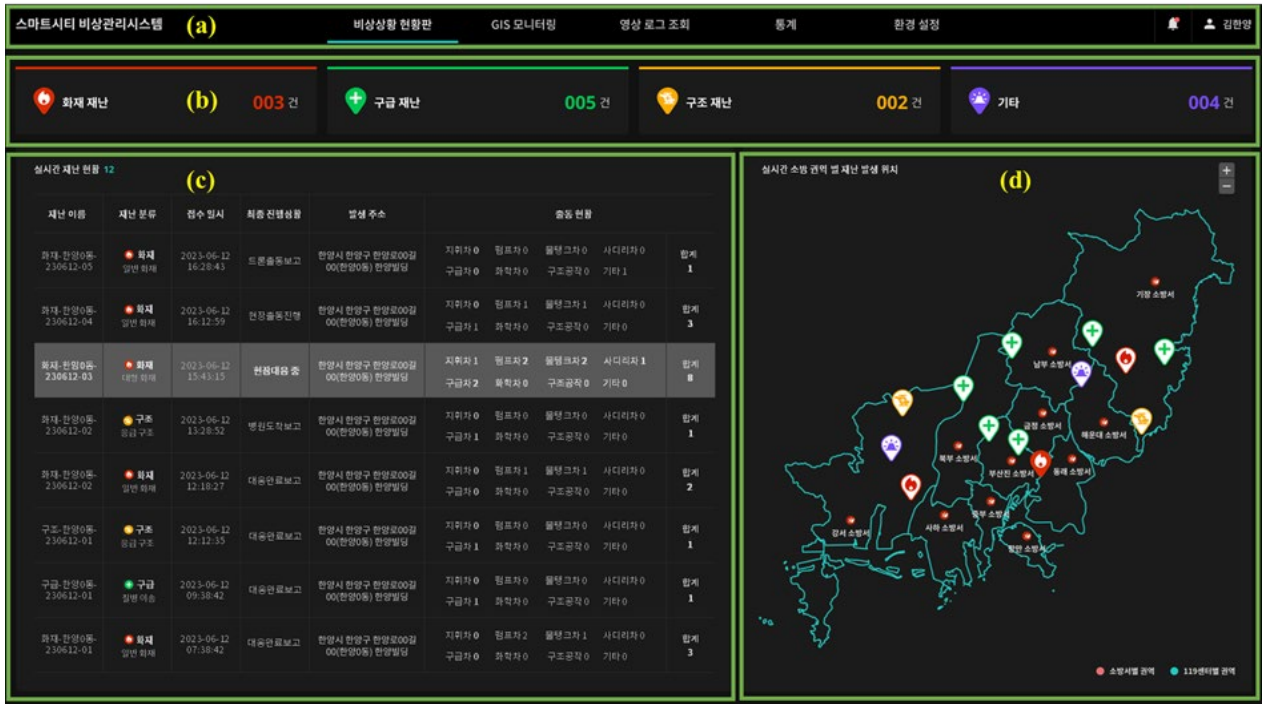
Fig. 2: Status dashboard configuration; (a) Global navigation menu for moving between menus, (b) number of occurrences by emergency type within a period, (c) real-time emergency information, (d) display location information via map chart
