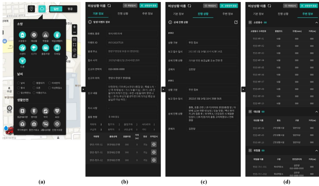
Fig. 5: Web-GIS dashboard map layer and right panel menu configuration; (a) various city information display layers, (b) emergency basic information, (c) emergency response progress information, (d) nearby facility information
