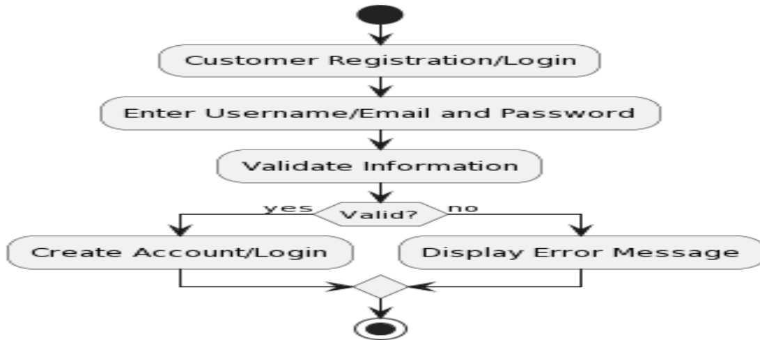
Fig 3: Customer login and registration diagram for the ARify's augmented reality e-commerce platform.
