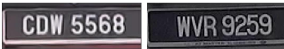
Fig. 5: A sample of a “comply” license plate (left) and a “not comply” license plate (right) due to \beta and \alpha that are too close.
