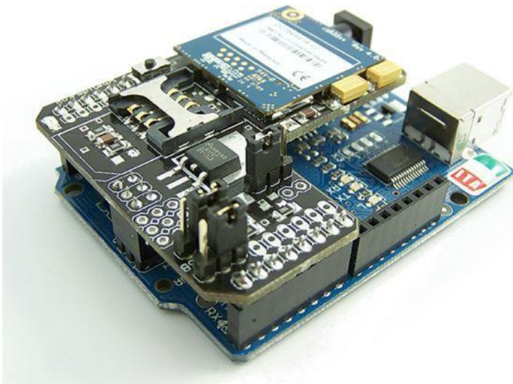
Fig. 1: GPRS Quadband module with SIM900 using Arduino
