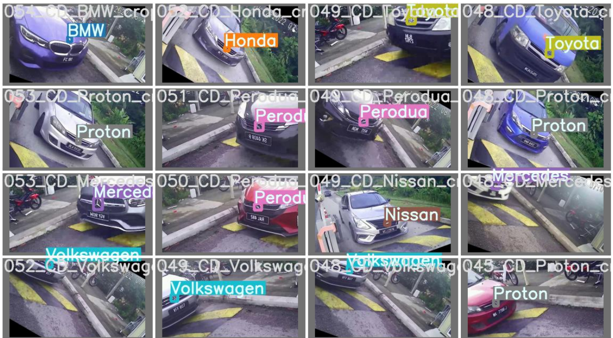
Fig.4: showcases the results of YOLOv7 logo detection using images captured under optimal lighting conditions.
