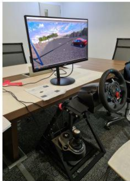
Fig. 1: The driving simulator prototype with a steering wheel rig.
