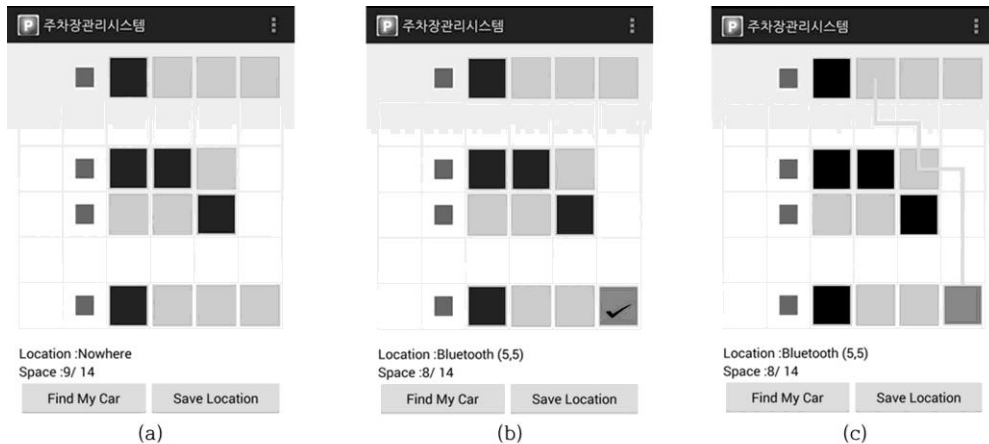
Fig. 8: User parking application: (a) saving the parking location, (b) current state of parking spaces, and (c) location guidance service.
