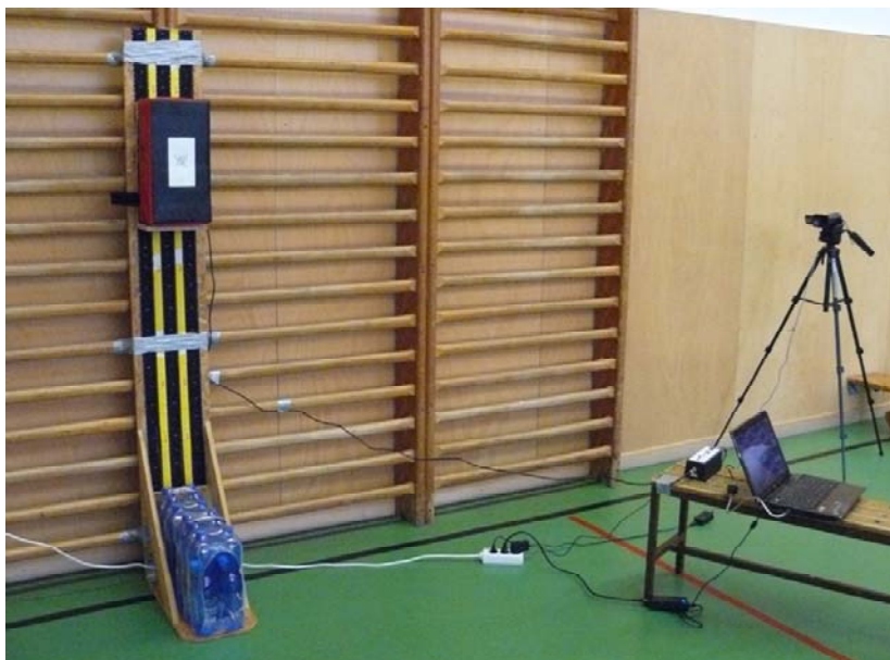
Fig. 8. Measuring station with sensor, computer and camera.
