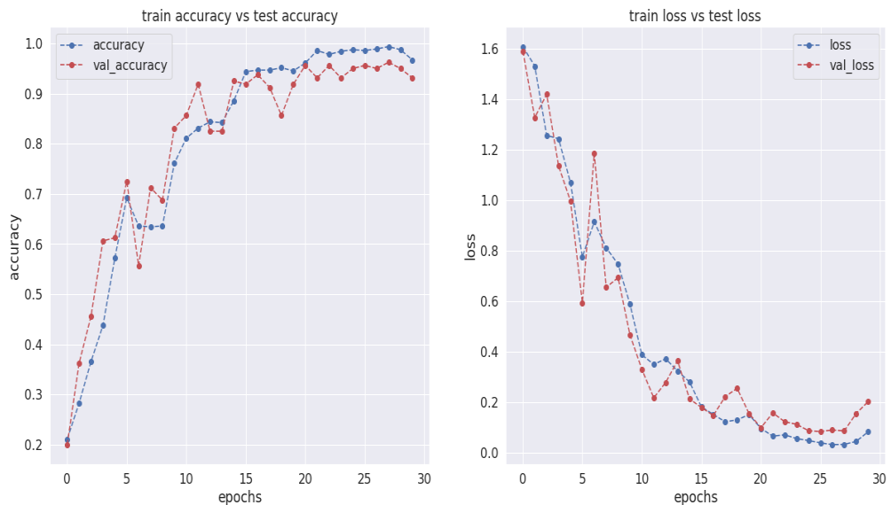
Fig. 2: Accuracy and loss of data training and testing of VGG16 proposed model
