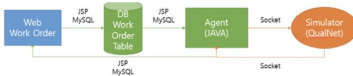
Fig. 12. Data Flow of WorkOrder Processing
